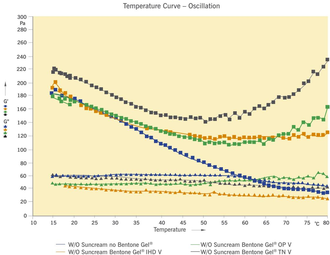
Figure 6. Formula 3 Oscillation Curve Over Temperature Range
