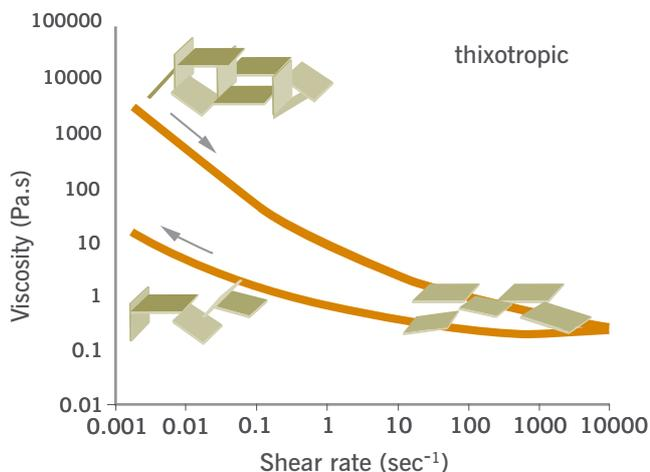
Figure 2. Hectorite Clay Flow Behaviour
